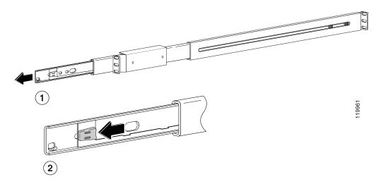
3. Using a screwdriver (1), gently press the button labelled "Push" and move the middle section of the outer telescopic rail to its end position, as shown in Figure 3-3.
